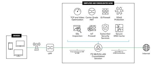
Figure 2: F5's N6 / S/Gi-LAN consolidated solution lowers CPU needs and simplifies automation, reducing CapEx and OpEx.
